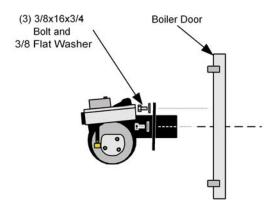
Figure 30. OWB-9, OWB-15 and OWB-25 Burner Mounting & Boiler Door Detail
